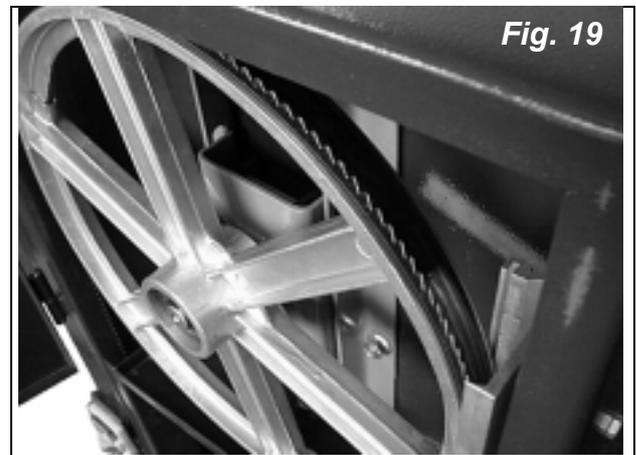
When the correct adjustment is achieved lock the tracking knob with the winged nut.
