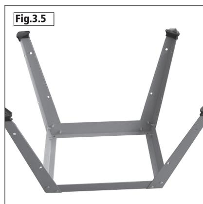
1. Feed the long fixing bolts up through the stand and secure the four corners using the washers and bolts provided **Fig.3.10**. Once this is achieved the whole stand can be fully tightened ready for the bandsaw to be fitted.
